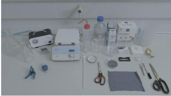
For the test, the textiles are cut into round pieces and stirred by magnetic mixers in a glass of liquid. After this process, the fibers are filtered and visually assessed.
